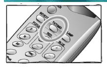
The **TXT/IMG** button allows you to switch between **Text** and **Image** settings. The **Text** mode increases the contrast by as set amount to improve the overall quality of text images. When in the **Text** mode, adjust the **Brightness** buttons to set the desired lighting for your text documents. In the **Image** mode, adjust **Brightness** to obtain the best results for full colored materials such as a
