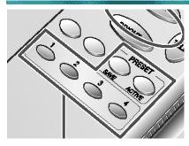
**PRESET** – Up to 4 User-defined presets can be stored allowing the presenter to quickly select up to four predetermined settings.
