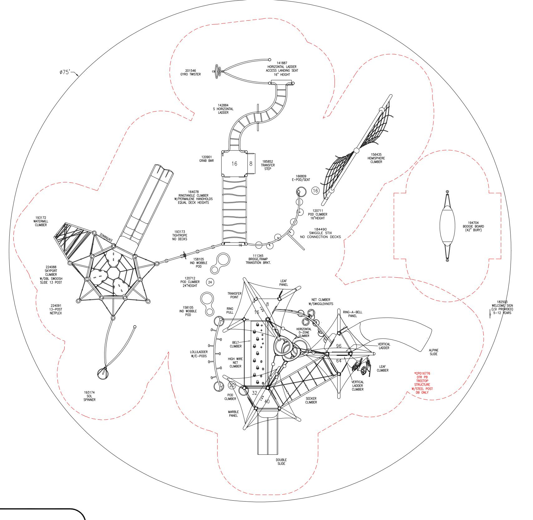
TOTAL ELEVATED PLAY COMPONENTS 14 TOTAL ELEVATED COMPONENTS ACCESSIBLE BY RAMP O <u>REQUIRED</u> O TOTAL ELEVATED COMPONENTS ACCESSIBLE BY TRANSFER <u>REQUIRED</u> TOTAL ACCESSIBLE GROUND LEVEL COMPONENTS SHOWN 17 REQUIRED 5 TOTAL DIFFERENT TYPES OF GROUND LEVEL COMPONENTS 8 REQUIRED 8
